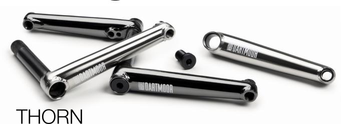
2-pcs design cranks made of heat-treated Cr-Mo 4130 steel with 22mm spindle and 48 splines. RHD/LHD compatible. Two sprocket holes to fit all sprocket sizes. Small gusset to make the pedals assembly area stronger. Includes arms, spindle (welded to the right arm), 2 spindle bolts (alu 7075-T6 and Cr-Mo), 2 sprocket bolts (bigger one is hollow) and assembly/disassembly tool.
