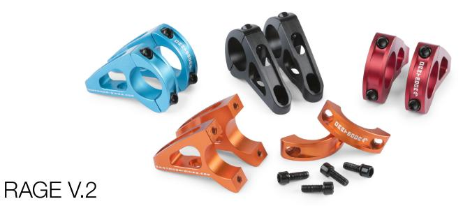
Upgraded version of our hi-end downhill stem with adjustable extension and re-designed body. Direct Mount standard for Boxxer, Fox or Dorado forks. Made of cold forged and CNC machined 7075 aluminium. We added to this stem a special washers securing the stem against changing its position when hitting the ground strongly.
