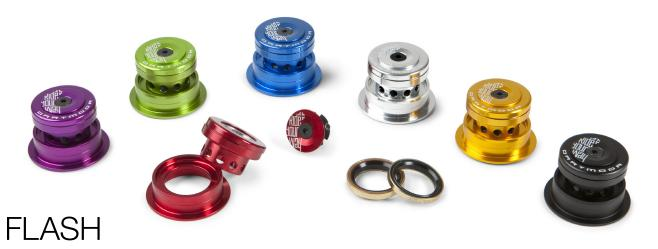
Top quality headset with external top part and zero stack (semi-integrated) bottom part. EC34/ZS49 type for tapered head tube and 1-1/8" fork steerer. Cups and top cover made of 2014 aluminium. Upper cup drilled for weight reduction with ultra low profile top cover. Bottom cup with integrated 1-1/8" reduction. High quality precision sealed 45/45 bearings with anti-rust titanium coating. Custom Ride Your Way compression cap included.
