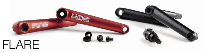
Light and strong 2.5-pcs cranks made of heat-treated Cr-Mo 4130 steel with 19mm spindle and 48 splines. RHD/LHD compatible. Two sprocket holes to fit all sprocket sizes. Small gusset to make the pedals assembly area stronger. Includes arms, spindle (pressed into the right arm), Cr-Mo spindle bolt, 2 sprocket bolts (bigger one is hollow), assembly tool.
