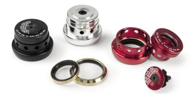
Top quality headset with external top and bottom parts. Cups and top cover made of 2014 aluminium. Both cups drilled for weight reduction. High quality precision sealed 45/45 bearings with anti-rust titanium coating. Custom Ride Your Way compression cap included. They come with two steel crown races, one for tapered and second for 1-1/8" forks.
