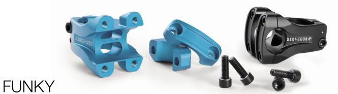
Our hi-end and unique stem made of cold forged and CNC machined 6061 aluminium. One of the lightest gravity stems on the market. Custom body shape with 2-pcs front plate design. All bolts are M6 size. Available in the full range of anodized colors: black, turquoise, green, red, blue, violet, gold and graphite plus silver polished and white coated.
