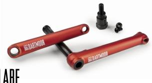
2.5-pcs design cranks made of heat-treated 100% Cr-Mo 4130 steel. Two sprocket holes to fit all sprocket sizes. Small gusset to make the pedals assembly area stronger. Includes arms, spindle (pressed into the right arm), spindle bolt (x1), sprocket bolts (x2), assembly tool.
