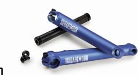
3-pcs design cranks made of heat-treated 100% Cr-Mo 4130 steel. Two sprocket holes to fit all sprocket sizes. Small gusset to make the pedals assembly area stronger. Includes arms, spindle, Cr-Mo spindle bolts (x2), sprocket bolts (x2), pinch bolts (x2). Alu spindle bolts available as separate spare parts.
