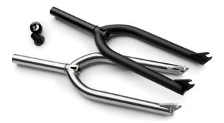
Lightweight park specific fork created for park/dirt riders. Designed to provide stability and control at high speed. Made of triple butted Cr-Mo 4130 steel. Post-weld heat-treated. Molded bottom section of the legs. 1-piece CNC machined steerer tube.
