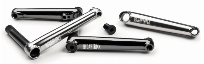
2-pcs design cranks made of heat-treated 100% Cr-Mo 4130 steel. Shorter spindle perfectly fits BMX frames. Two sprocket holes to fit all sprocket sizes. Small gusset to make the pedals assembly area stronger. Includes arms, spindle (welded to the right arm), spindle bolts (x2), sprocket bolts (x2), assembly/disassembly tool.
