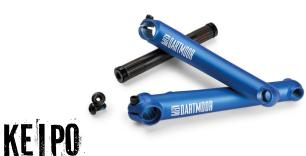
3-pcs design cranks made of heat-treated 100% Cr-Mo 4130 steel. Two sprocket holes to fit all sprocket sizes. Small gusset to make the pedals assembly area stronger. Includes arms, spindle, Cr-Mo spindle bolts (x2), sprocket bolts (x2), pinch bolts (x2). Alu spindle bolts available as separate spare parts.
